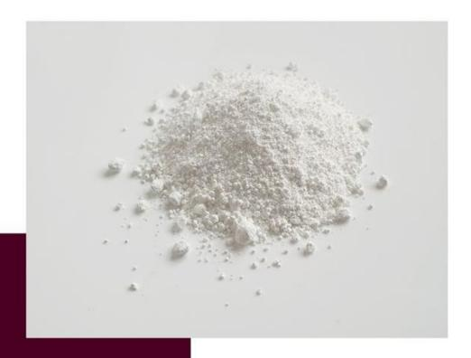
Sodium chlorite is a chemical compound with the formula NaClO2. It is a white crystalline solid, odourless and non-flammable. It is used in water treatment, industrial processes, and food preservation. It is often used as a disinfectant due to its ability to kill a wide variety of microorganisms and eliminate odours. Sodium chlorite can be used to disinfect drinking water, swimming pools, and wastewater. It is also used in medical and dental settings to clean equipment and surfaces.
