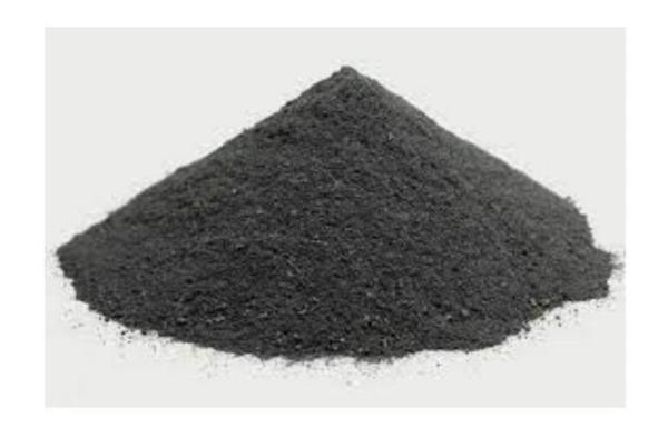
Tantalum is a rare transition metal that is mined from columbite-tantalite, which is an ore found in various parts of the world. The metal is particularly known for its high melting point and its resistance to corrosion, making it an ideal choice for many applications in a wide range of industries. It is also known for its excellent conductivity, malleability, and ductility, as well as its ability to form strong bonds with other materials.
